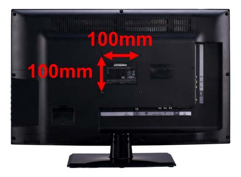
Mounting Specification: **100mm x 100mm** using screw size **M4**. Length of screw should not exceed **6mm**. Please Note: The **6mm** length of screw refers to how deep the screw can go inside the mounting holes. When you're buying screws, you should add the original 6mm to the thickness of your mounting plate in order to get the total screw length.
