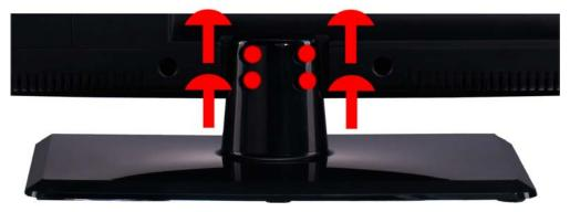
2. T o attach the stand place the display unit flat on a table. Afterwards attach the stand onto the display and screw in the 3 screws to secure the stand.
